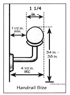
R311.5.6.3 Handrail grip size. (675 IAC 14-4.3-30) The handrail grip size portion of handrails shall have a circular cross section of 1½ inches minimum to 2-7/8 inches maximum. Other handrail shapes that provide an equivalent grasping surface are permissible. Edges shall have a minimum radius of 1/8 inch.
